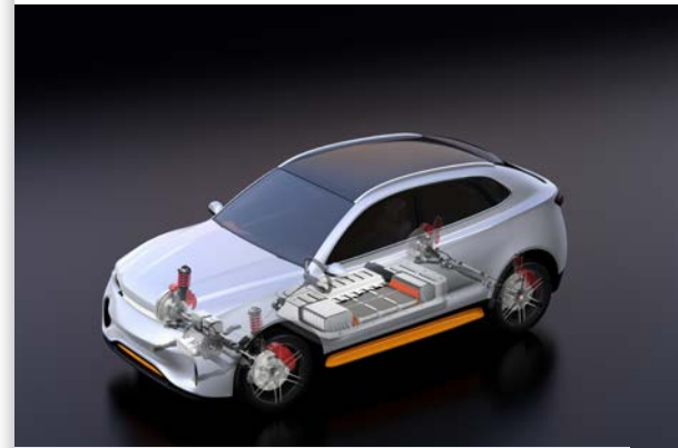
Lithium battery pack in an electric car
