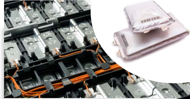
Electric car lithium battery pack and wiring
