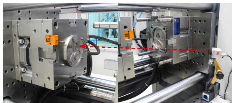
Positioning the infrared camera in the tool installing area
